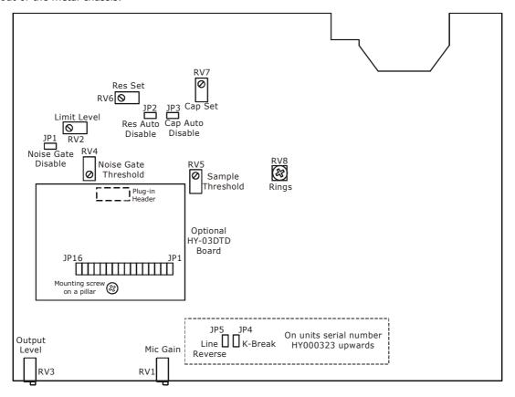
Figure 1-3: HY-03 Preset Controls and Alignments
