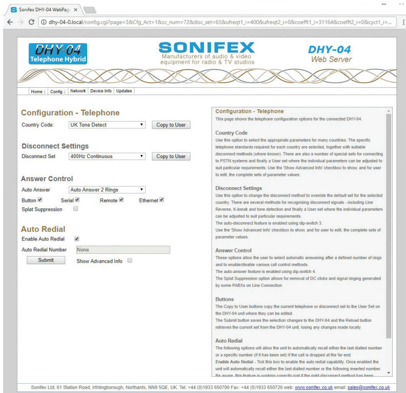
Figure 6-5: Telephone Configuration – selection of telephone interface via Country Code selection.
