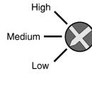
The level of the input received by the unit depends on which of the three settings is selected. With the switch set to low, a -12dB signal received is output at 0dB. Selecting the Medium or High settings add +6dB and +12dB to the level respectively. Set the level so that the meter readings peak at the 0dB scale mark.
