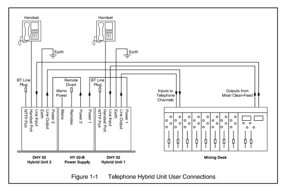
The telephone line NTTP port may be directly connected using the BT 6/502 cable mounted connector into a suitable BT wall jack socket. A simple telephone handset can be used to take and make calls when plugged into the equipment handset connector BT 605A. Some versions of this equipment will be supplied with variations of the telephone line or handset connectors.
