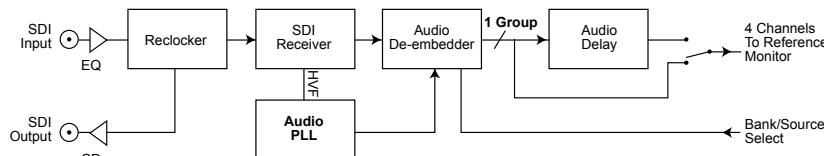
Fig 3-2: RM-HD1 Block Diagram
