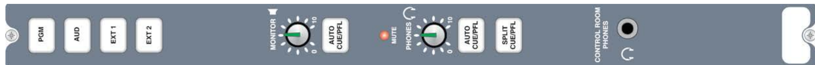
S2-OMC Control Room Monitor Channel.
