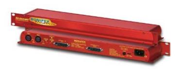
The RB-DA24MD has two XLR inputs and up to 24 outputs on a pair of D-subs. A release explains that it has "two inputs which can be individually routed to 12 outputs or mixed and routed to all 24 outputs. The inputs can be configured as either dual-mono, Input 1 routed to outputs 1–12 and Input 2 routed to outputs 13–24, or mixed-mono, Inputs 1 and 2 mixed at a preset level and routed to all 24 outputs."
